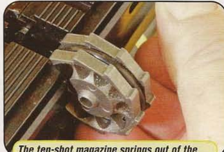
The ten-shot magazine springs out of the breech when you move the brass bolt, which makes loading and unloading very easy
